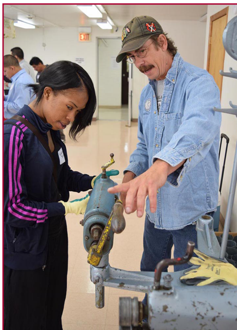
Sheet Metal Local 73 Instructor Ron Kaps demonstrates to this woman how this piece of equipment prepares a duct connector collar.
